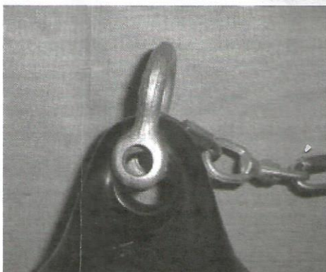
Push shackle down over eyelet.
